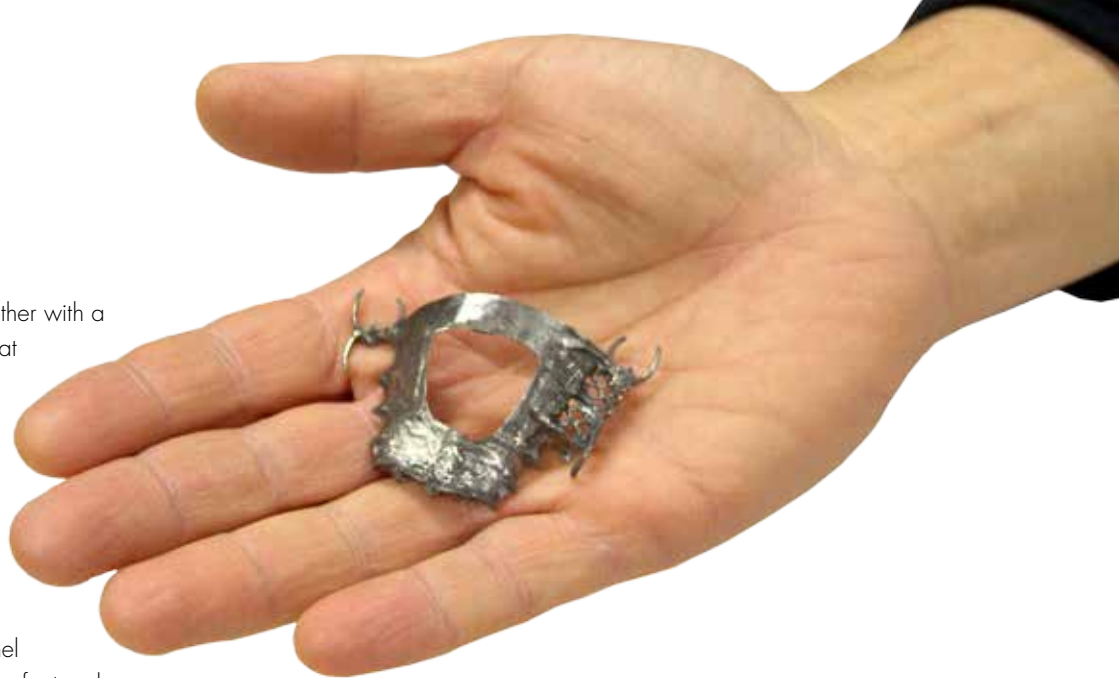
A 3D printed partial denture plate that is undergoing continued refinement and testing as part of Dr. Ference and Dr. Chmielus' research.
